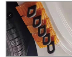
2. Apply hot melt glue on the pull tab and stick it to the place that needs to be repaired.
