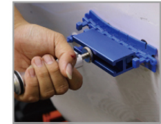
2. Install the slide hammer on the adapter fitting and carry out the repair work.
