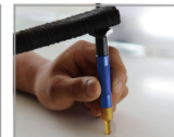
2.Aim the tapping pen at the raised part and tap it to make it flat.
