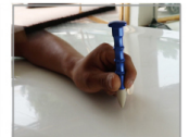
2.Aim the tapping pen at the raised part and tap it to make it flat.
