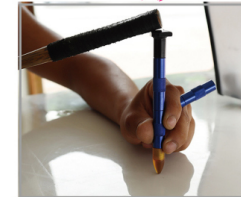
2.Aim the tapping pen at the raised part and tap it to make it flat.
